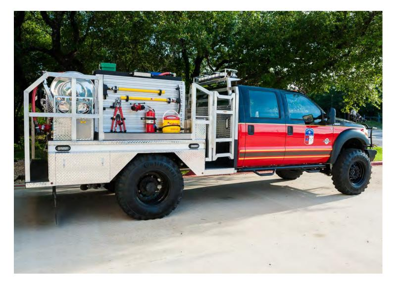
Brush Trucks are designed to move quickly through areas that other fire apparatuses cannot. They can store up to 400 gallons of water and can be used for light rescue, initial attack or medical support. Our trucks are also equipped with a remote controlled nozzle, which enables the vehicle to fight fire on the move.
