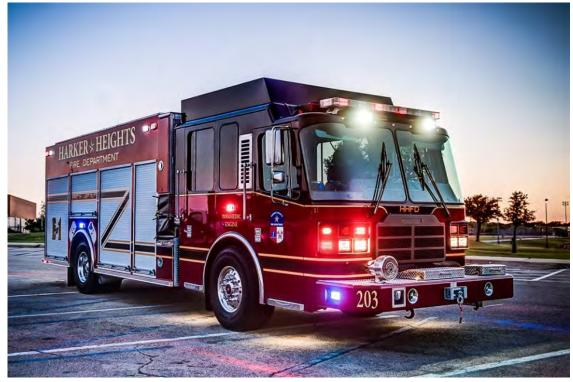
Engine 1 is a 2014 Ferrara MVP Pumper Truck. It can store up to 750 gallons of water and pump 2000 gallons per minute. It carries up to 768 cubic feet of equipment. The truck is approximately 34' long and 10' in height.
