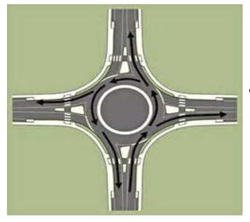
Although the picture to the left is <u>not</u> the design for Commercial Drive, it provides an idea of what a roundabout is and how it functions for traffic flow.
